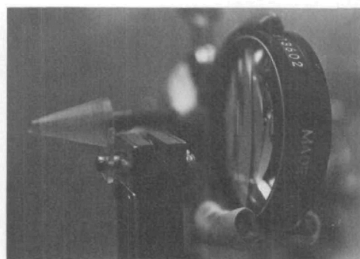
Fig. 1A. Isometric force-displacement transducer with applanating lucite cone and 20 diopter lens for the measurement of episcleral venous pressure.
