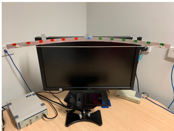
FIGURE 1. A metal arc mounted to the top edge of the monitor with targets at ± 30 degrees from the center in 5-degree steps. It was used to measure the gaze position of the subject.
