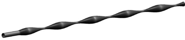
Figure 4. Tunnel shape (modulated radius) used in Experiment 2. The total length of this tunnel is 1147 m, but different lengths were also used (see text). For better visibility, the radius is exaggerated by a factor of 3.
