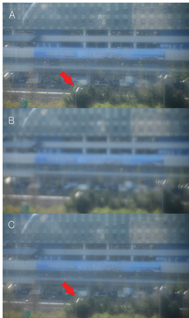
Figure 9. Focusing with bifocal IOL. (A) With the bifocal IOL, the image was hazy and foggy compared to the monofocal IOL when the first (far) focus is on the focal plane of the objective lens, and the halo (diameter: 171 pixels) is observed around the street lamp ( arrow ). (B) As the cornea-IOL complex approached the focal plane of the objective lens, the image became significantly blurry. (C) Then, it became clear again when the second (near) focus was on the objective lens. At this time, the halo (diameter: 203 pixels) was observed around the street lamp ( arrow ).
