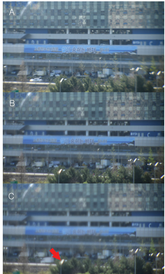
Figure 8. Focusing with Eyhance. (A) With Eyhance, when the far focus was on the focal plane of the objective lens, the image was clear. (B) As the cornea-IOL complex approached the objective lens, the image became slightly blurry. (C) Then, it became slightly clearer again. At this time, a halo was observed around the street lamp, which was small (diameter: 60 pixels) but strong (arrow). There was a clear image of street lamp by the second focus of Eyhance inside the halo.
