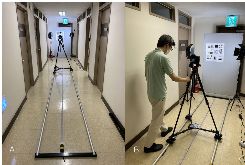
Figure 4. Experiment set up for quantitative analysis. (A) We printed the USAF 1951 resolution test target on 50 cm × 50 cm paper and attached it to a stand panel. Two LED lights (GVM 800D-RGB LED Studio 2-Video Light Kit) were used to illuminate the target at an angle of 45° each. A video of the mobile model eye approaching the target from 6 m to 15 cm was recorded. A dolly track (Glide Gear, Straight Track with Carry Bag [12]) was installed on the floor for film shooting. A tripod dolly with wheels (Glide gear, tripod dolly SYL-960) was put on the track. A tripod was installed on the tripod dolly. (B) A mobile model eye was installed on the tripod. A tape measure was installed on the floor and inside the dolly track. An additional camera (iPhone 4) was installed on the tripod dolly to record the tape measure on the floor. During the recording, the dolly was pushed as the researcher walked.
