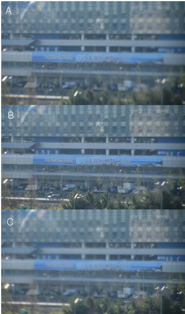
Figure 7. Focusing with monofocal IOL. With monofocal intraocular lens, the letters on the signboard were clearly visible when the focus was on the focal plane of an objective lens. However, they became blurry as the focus passed the focal plane of the objective lens. (A) The focus of the monofocal IOL in front of the focal plane of objective lens. (B) The focus of the monofocal IOL at the focal plane of objective lens. (C) The focus of the monofocal IOL behind the focal plane of objective lens. The focus of the monofocal IOL was 0.44 mm closer to the focal plane of objective lens than panel A.
